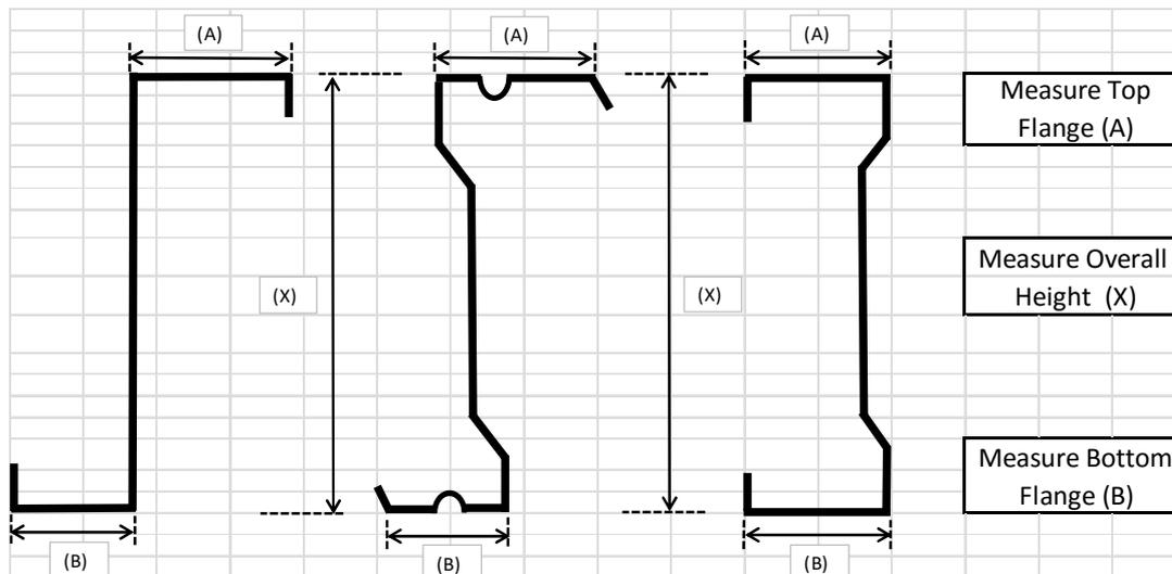
Most Purlins are stamped or identified with the manufacturer's Code or Part Number and this is sufficient for identification purposes. Should there be any doubt as to which purlin is being used please contact our Technical Sales Staff who can assist in identification to ensure the correct clip is ordered and supplied
